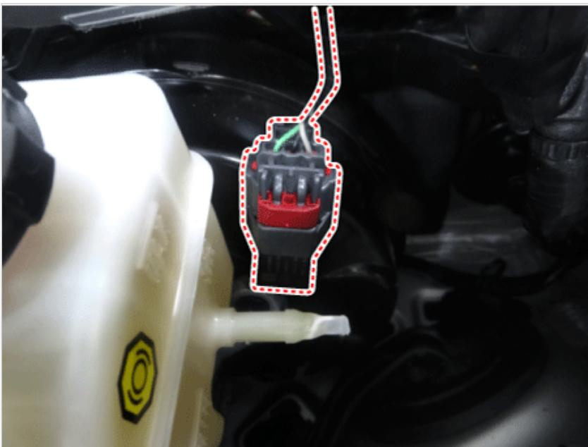
10. Disconnect the brake vacuum hose (A) and brake fluid level sensor connector (B).
